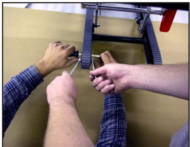
Figure 36 - Tensioning the Belt
