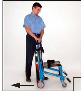
**Figure 8 - Aligning the Wheels**
