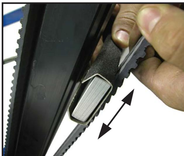
**Figure 40 - Sand in Direction of Arrows**
