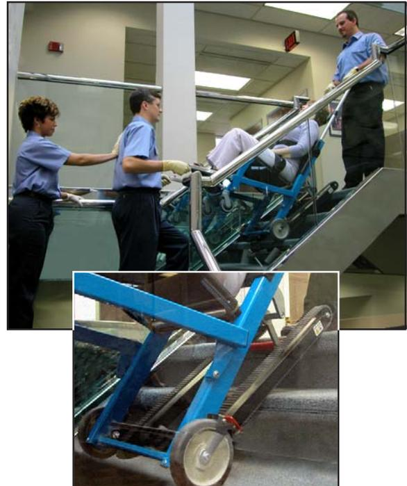
Figure 25 - Establishing the Glide Angle
