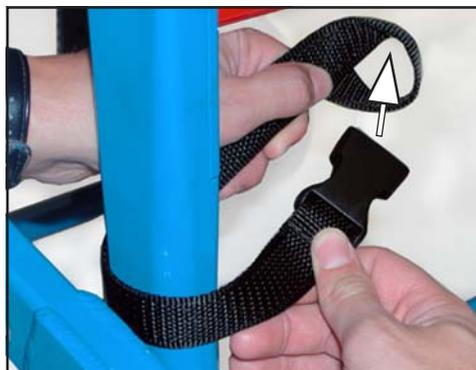
**Figure 4 - Threading Buckle Through Loop**
